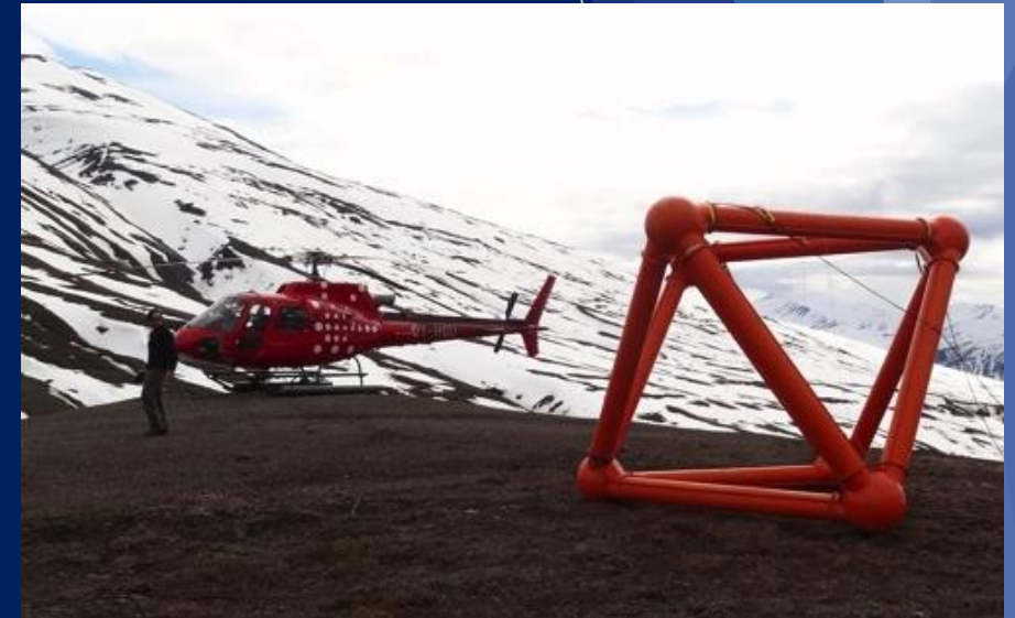
2012 helicopter-borne ZTEM survey at Kangerluarsuk
